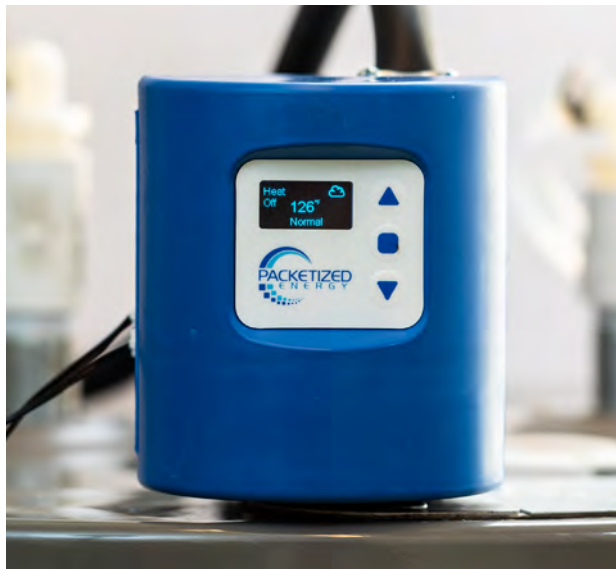
The Mello, a small device that fits on top of an electric resistance water heater, optimizes when the heater runs.
